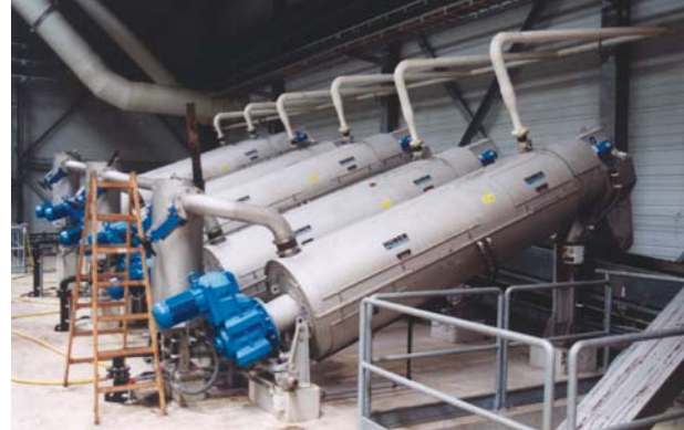
Digested residue is pumped to the solids dewatering unit, where a flocculant/polymer emulsion is added before material goes to screw presses.
